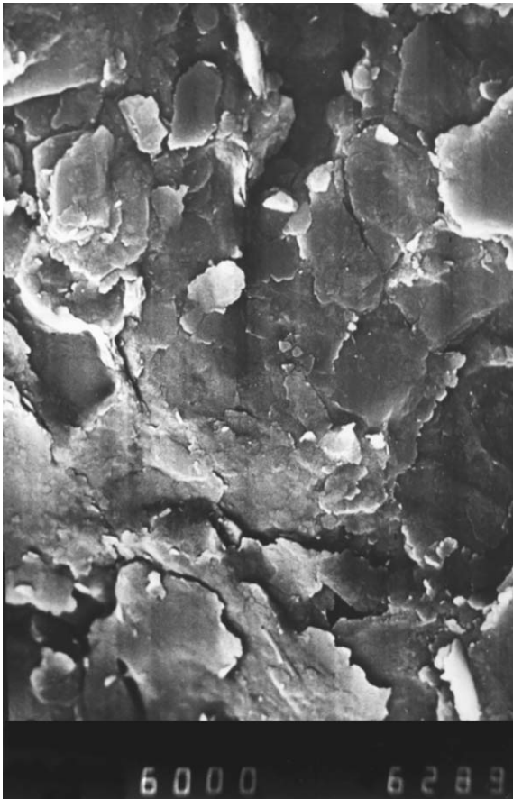
Fig. 11. Scanning electron micrograph of Fithian, Illinois illite.
