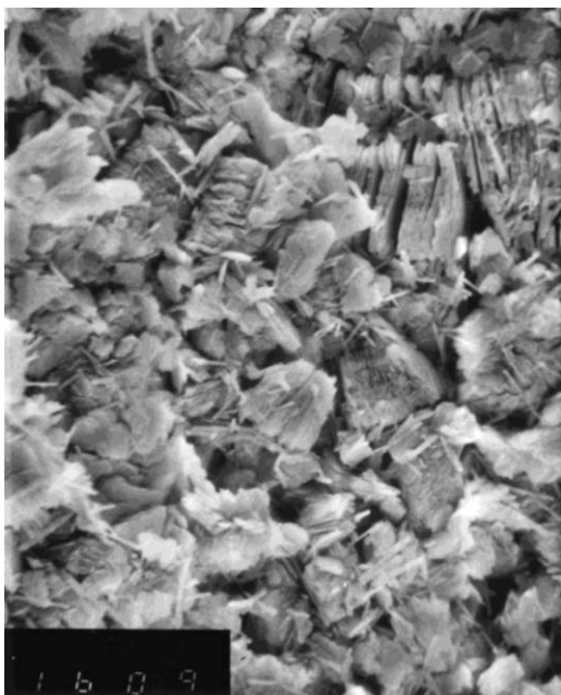
Fig. 32. Scanning electron micrograph of Belitung kaolin.
