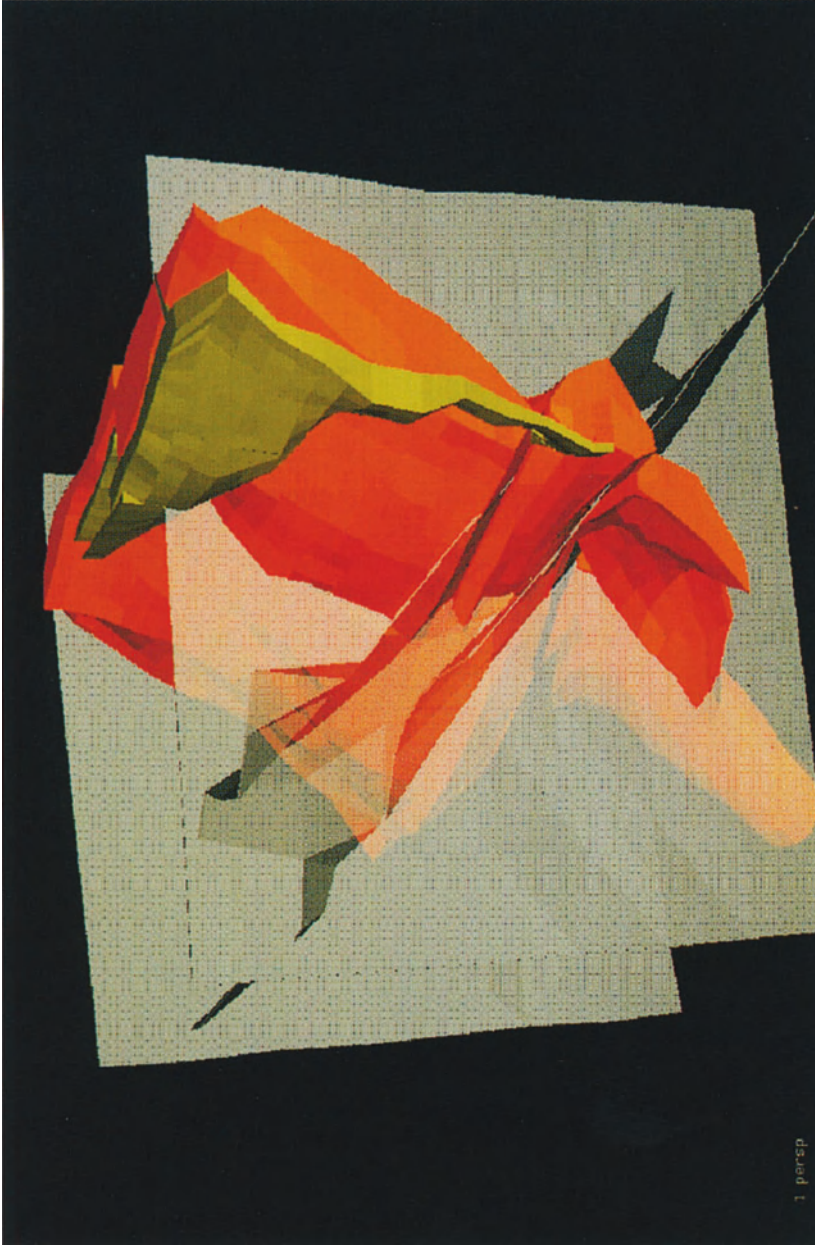
Fig. 2.1 3D view of a computer representation of an inclined mineral ore deposit with intruding basalt dikes (olive green) and multiple fault discontinuities; fault surfaces are shown semi-transparent
