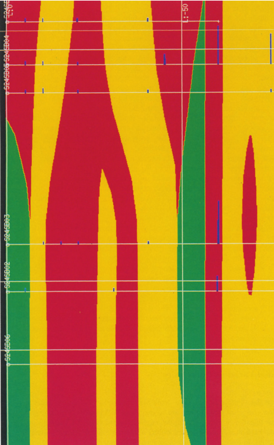
Fig. 2.2 Viewplane section through a 3D model of sedimentary soil geology with contaminant sample information from borehole investigation overlaid in histogram format
