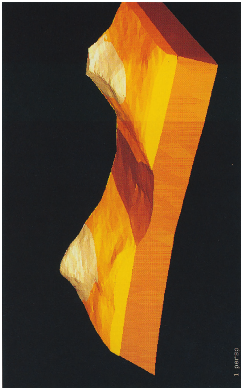
Fig. 7.10 Volume model representation of faulted, eroded stratigraphic units that outcrop at topography, truncated by a near-vertical fault surface in the foreground; generated from the composite surface information shown in Fig. 7.8 and Fig. 7.9
