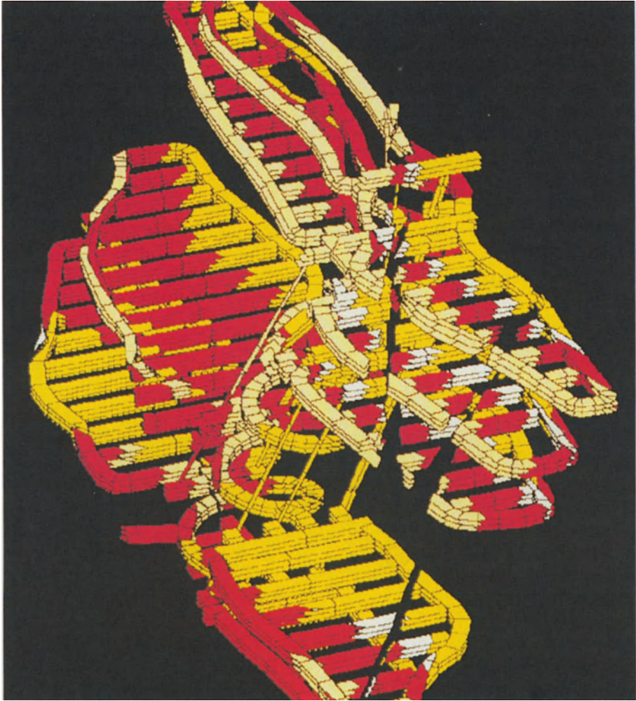
Fig. 13.8 3D visualization of the volumetric intersection of mine development and stoping excavations with the volume model representation of mineralogical ore types within the deposit; ore type CBO is brown , MBO is red , MYO is gray and PYO is yellow ; gaps in the ore deposit intersection are caused by the barren intrusive dikes
