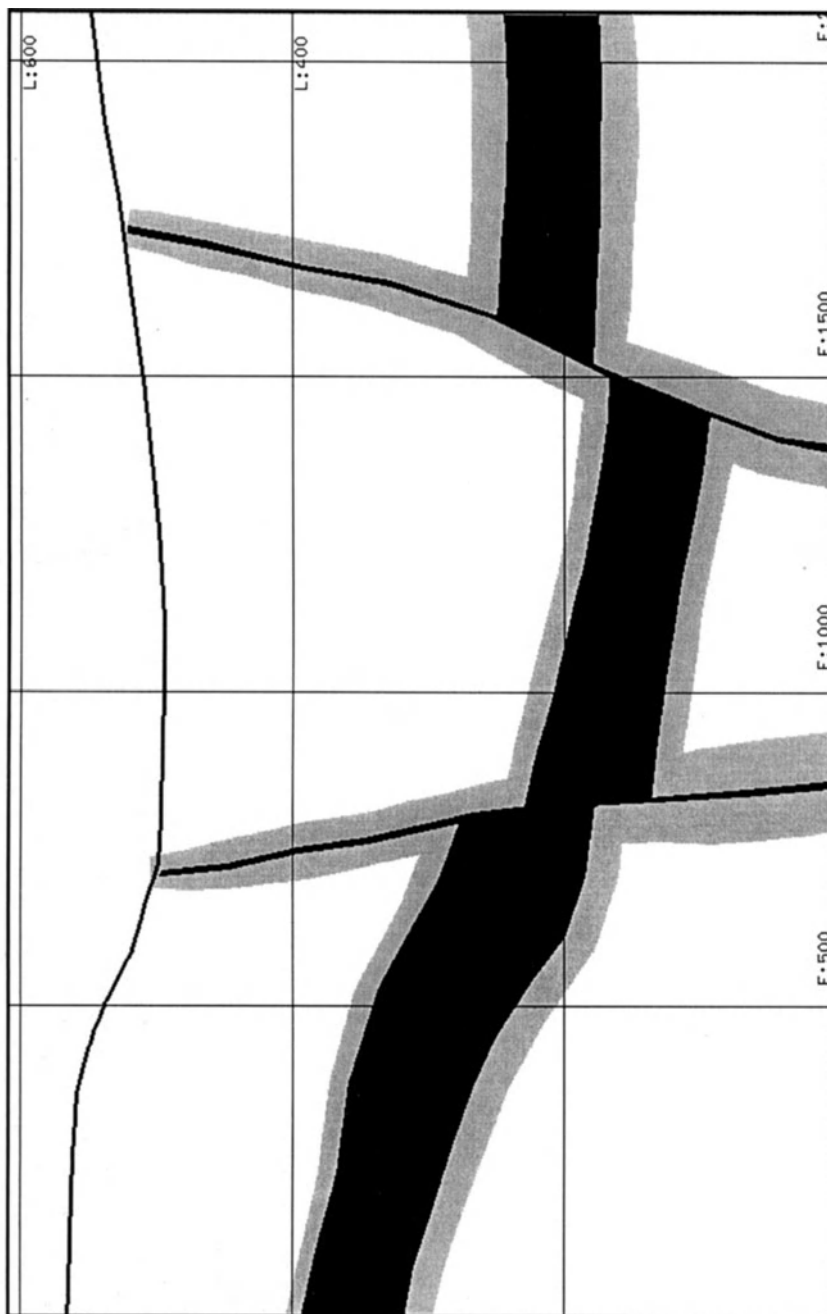
Fig. 10.5 Viewplane section through a volume model representation of topography, fault surfaces and faulted strata ( dark gray ); fault and strata surfaces have been determined by geostatistical prediction; the extent of the resulting locational uncertainty is light gray
