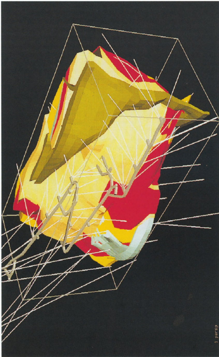
Fig. 13.4 Detailed 3D interpretation of mineralogical ore types within the deposit; dark green intrusions in right foreground are basalt dikes
