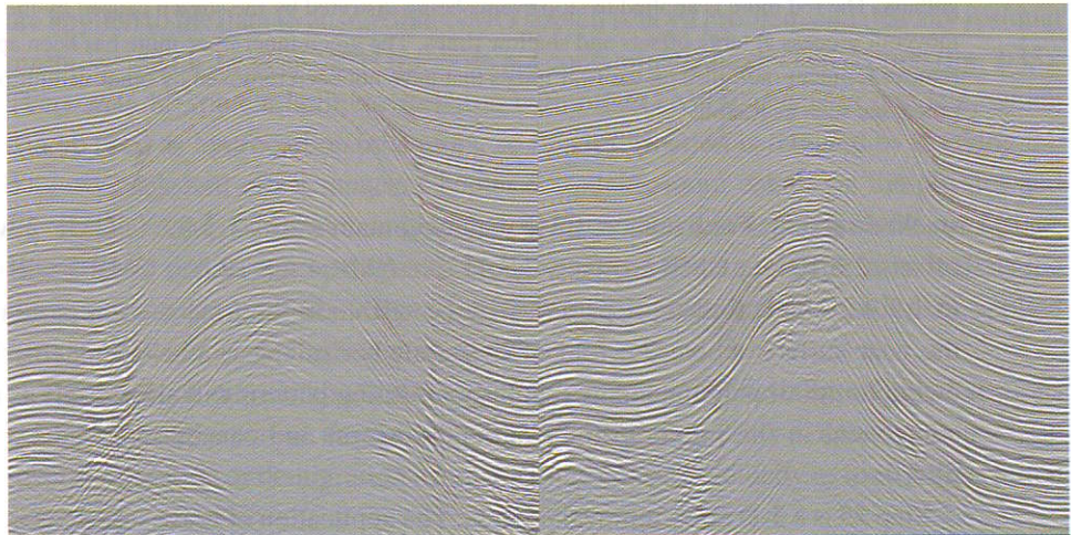
Fig. 2.36 Example of seismic data before and after migration. Data on the left are unmigrated, on the right they are migrated. Notice how the migration process has reduced the apparent size of the structure. Note also that whereas the picture on the left has reflections that cross each other, those on the right are geologically consistent.
