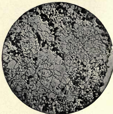
FIG. 108.—CHALK, ALTERED BY DOLERITE. Scawt Hill, Co. Antrim, Ireland. Shewing Wollastonite, Zoisite, Scapolite, and Magnetite in clear Calcite. × 25 diam.
