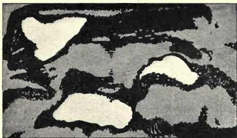
FIG. 114.—OCCURRENCE OF CORUNDUM. Tuli district, Rhodesia. ( About half scale ). Feldspathic Matrix, shaded; Magnetite and Spinel, black; Corundum, light.
