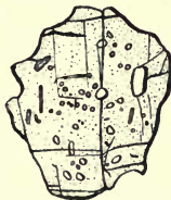
FIG. 5.—GARNET, IN GNEISS, showing the dark margins and pitted appearance due to a high refractive index, and the inclusions characteristic of metamorphic rocks. Near Limpopo River, Transvaal. \times 20 diam.
