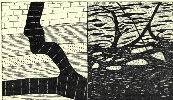
FIG. III.—Shewing contrast between contacts of dykes and deep-seated rocks. (Igneous rocks black.)
