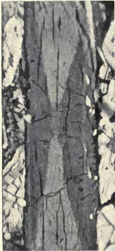
FIG. 32.—AUGITE. Longitudinal Section, showing hour-glass Zoning. \times 40 diam. In nepheline dolerite of Lobauer Berg, Saxony.
