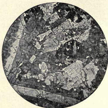
FIG. 80.—COARSE GRANULAR DOLERITE. Scawt Hill, Co. Antrim, Ireland, \times 15 diam. (From Geological Magazine , after Gough).
