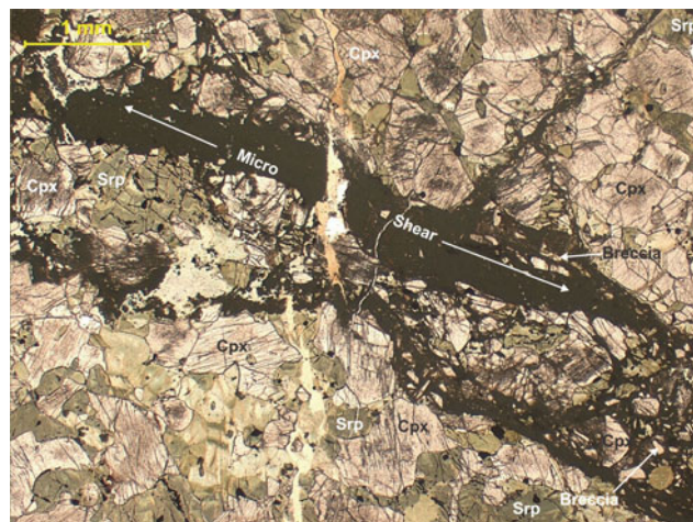
Plate SP-15 Micro-shear in spinel lherzolite containing pulverised and brecciated grains of clinopyroxene and serpentine (96/80b)
