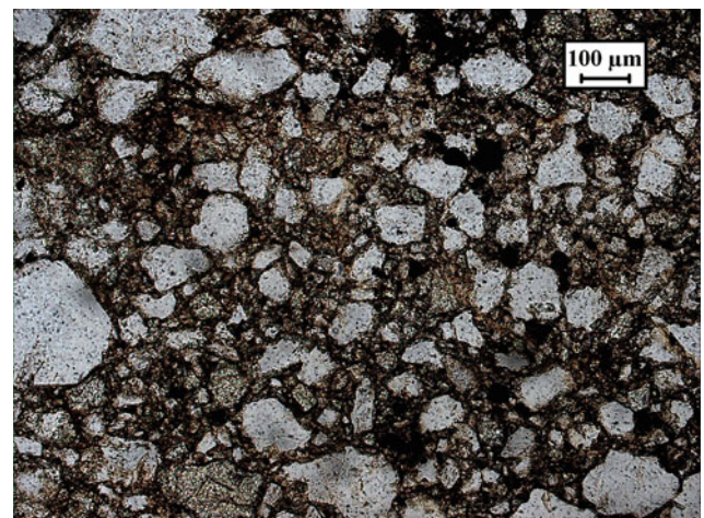
Plate Py-19 Volcanic tuff breccia between crossed polars containing angular rock fragments (124-79-7)
