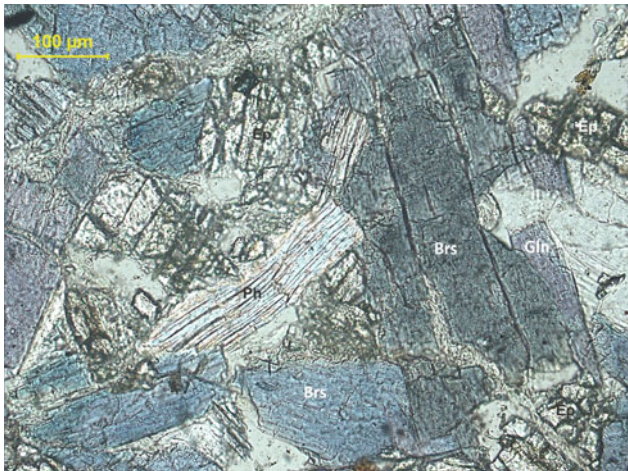
Plate Ec-13 Large flakes of phengitic mica in association with barroisite/glaucophane and epidote in eclogite (77/80-4)
