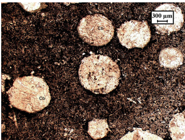
Plate V-66 Amygdaloidal basalt containing vesicles filled with devitrified glass and carbonate (calcite) (B69)
