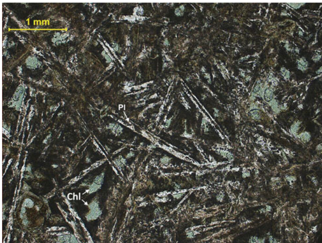
Plate V-56 Radiating laths of plagioclase and chlorite pseudomorphs after pyroxene in basalt showing intersertal texture (567/78-1)
