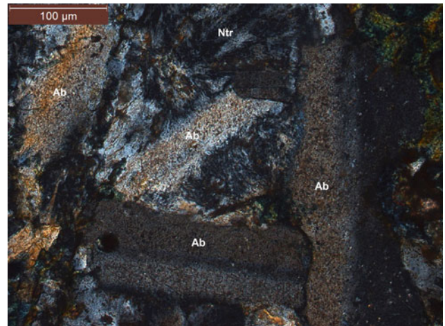
Plate Vlgm-4 Intergranular texture in epidote-chlorite-natrolite-albite rock between crossed polars (K-79-1)
