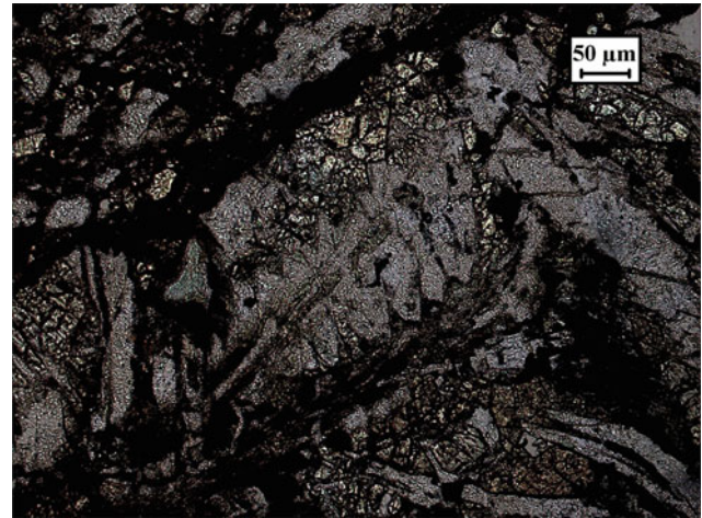
Plate Hy-13 Magnified view of dog-tooth augite with serrated margins in glassy groundmass of hyaloclastite (37/79-1). Brown granular clinopyroxene altered to chlorite occupies the interstitial spaces between the plagioclase grains (37/79-2a)
