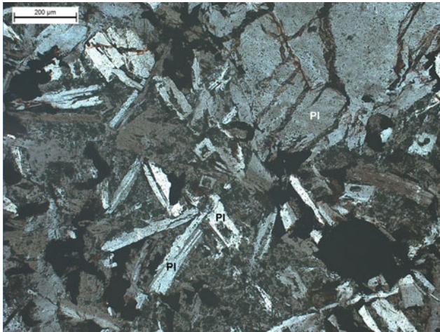
Plate Hy-15 Magnified view of the contact in basalt 26/79-3 showing laths of randomly oriented plagioclase in a glassy groundmass (26/79-2)
