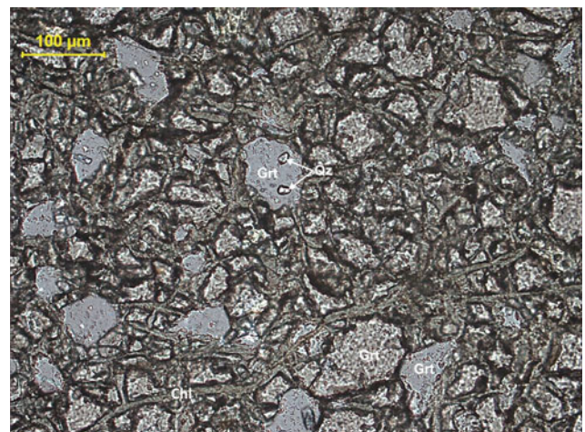
Plate Ec-3 A portion of a large, highly resorbed garnet porphyroblast in eclogite showing secondary chlorite veins cutting through islets ( pieces ) of the original garnet containing quartz inclusions (77/80-7)
