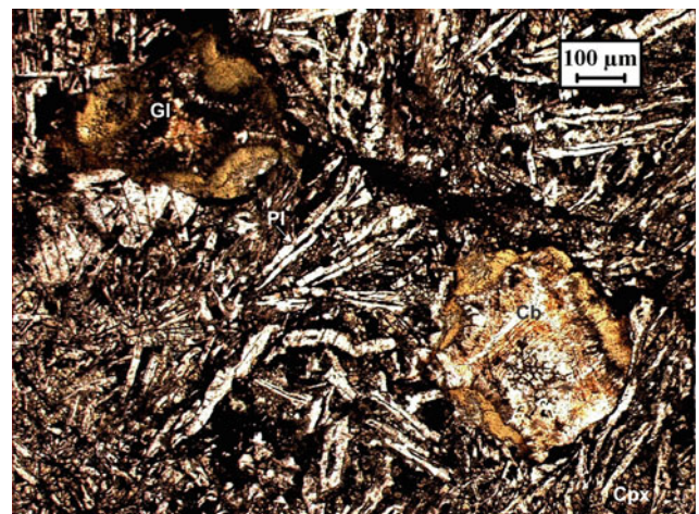
Plate Hy-18 Hyaloclastite 37/79-1 fragments with clasts of yellowish brown carbonate surrounded by curved plagioclase and intergranular pyroxene. The carbonate is rimmed by brown palagonite glass (37/79-3)
