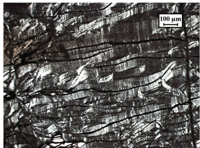
Plate S-4 Ribbon texture in serpentinite between crossed polars (192/80)
