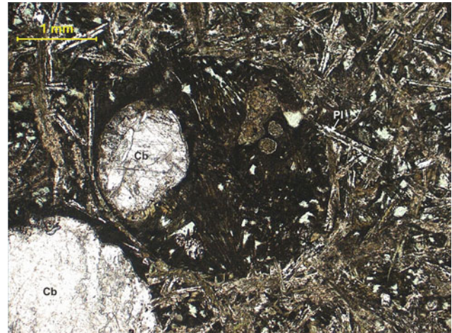
Plate V-57 Amygdaloidal basalt with carbonate-filled vesicles and acicular needles of plagioclase and mafic minerals (epidote) within the vesicle. The host basalt shows an intergranular texture (567/78-3)
