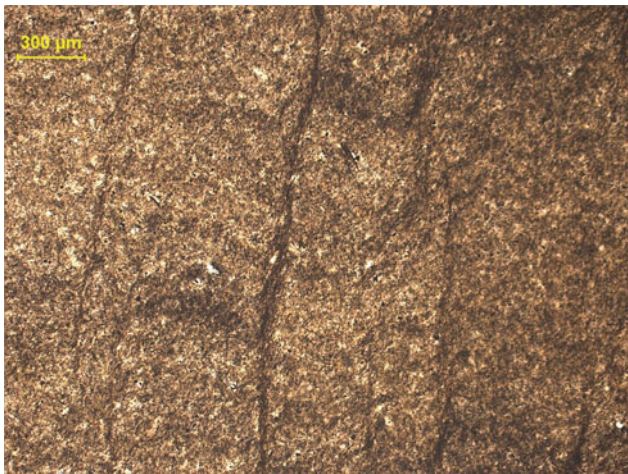
Plate OS_T-1 Pressure solution fracture in tuffaceous sediment. Slippage and plastic flow developed by ino-silicates under stress such that the strain is limited to a secondary fabric (507/79-1)
