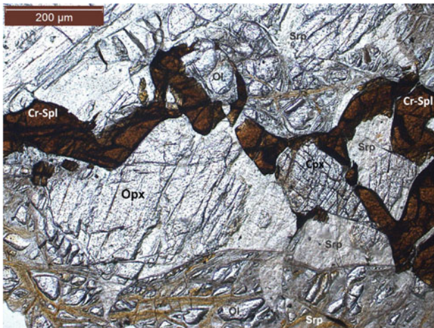
Plate SP-5 Coarse, protogranular harzburgite containing olivine remnants traversed by serpentine, large crystals of non-pleochroic orthopyroxene and skeletal Cr-spinel. Both serpentine and orthopyroxene are trapped within spinel on right . The spinel band on left is flanked by orthopyroxene on either side (R-16-5)
