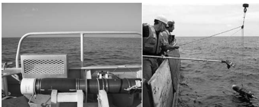
Fig. 17.2. A SOLO underwater float equipped with a hydrophone (left) being launched for testing (right). Photo courtesy Frederik Simons.
