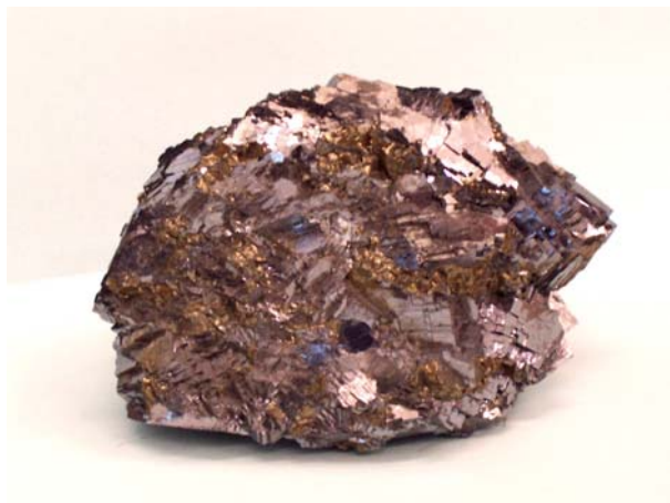
Fig. 2 An example of coarse, cubic galena (PbS), the principal ore mineral of lead, intergrown with pyrrhotite (iron sulphide). Sample taken from Black Mountain Pb-Zn-(Cu-Ag) mine in the northern Cape Province, South Africa.
