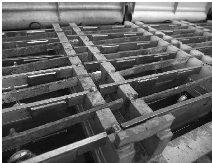
Fig. 10. Electrolytic cells showing the titanium cathode plates.
