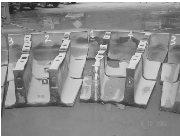
Fig. 6. Pulp lifter wear demonstrating slurry backflow.
