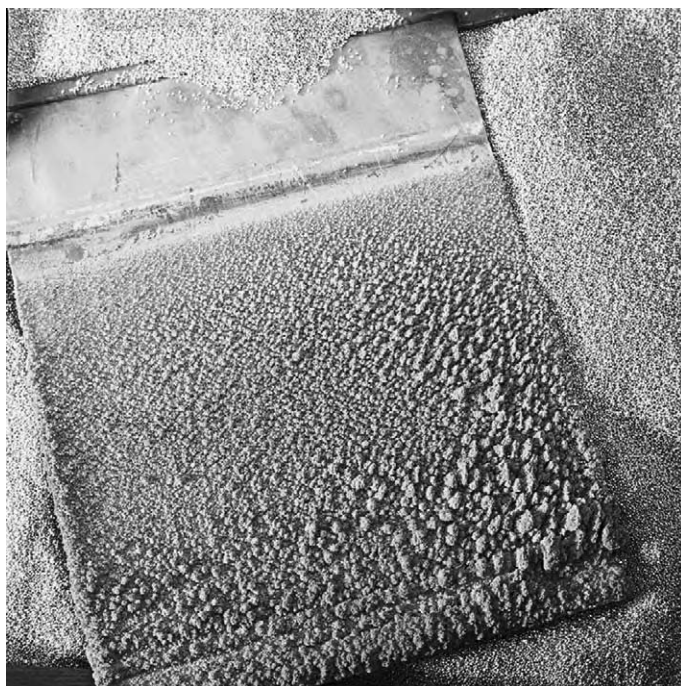
Fig. 9. 9999s sponge gold on a cathode plate.
