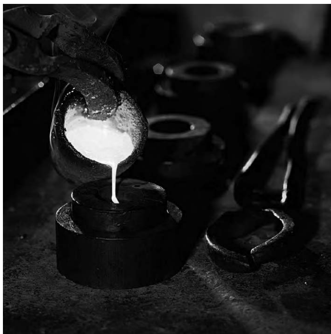
Fig. 4. Pouring a gold button prior to analysis by fire assay.
