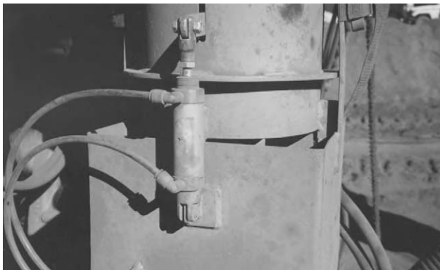
Fig. 2. Incorrectly designed sample divider on the side of a drill rig that collects material from only one side of the stream of cuttings (see slots on right-hand side of rectangular sample division device).
