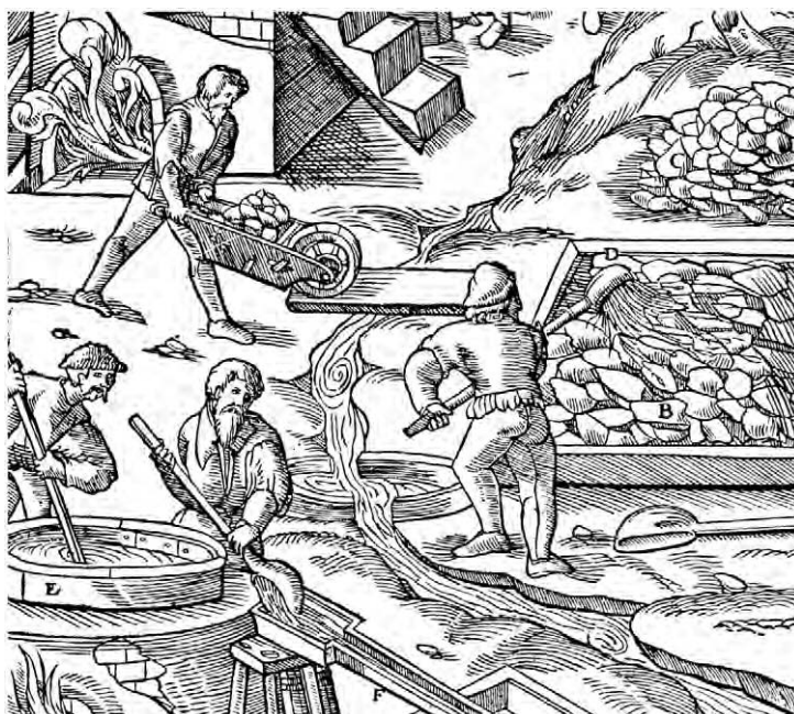
Fig. 1. “The rocks are . . . piled in . . . heaps fifty feet long, eight feet wide and four feet high, which are sprinkled for forty days with water. The rocks begin to fall to pieces like slaked lime, and there originates a . . . new material”. (Drawing and text from De Re Metallica ; Agricola, 1556).
