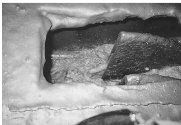
Fig. 6. Shark-fin cutters are unsatisfactory sampling devices, because they do not take a full cross-section of the slurry stream.
