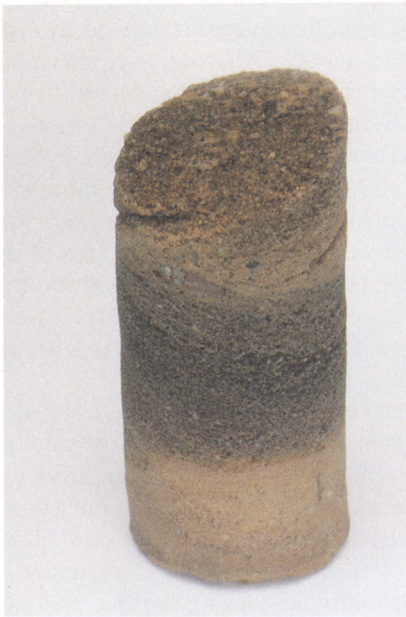
Fig. 2. Core cut from an outcrop sample from the Triassic Burghead Beds, Burghead, north-east Scotland. The cross-bedding in the core sample (a) is also clearly visible on the unwrapped permeability image derived by 4 mm grid sampling on the outer surface of the core cylinder (b).
