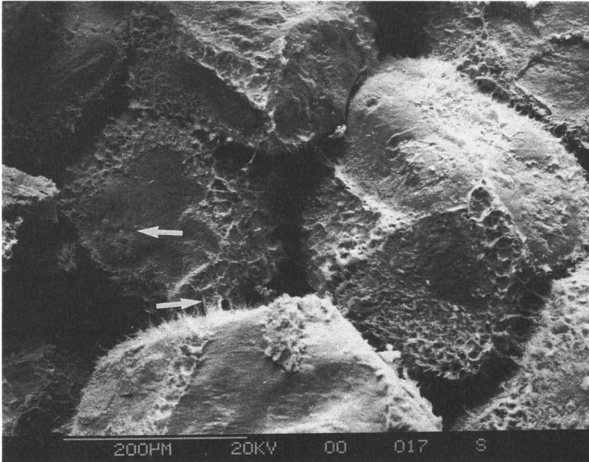
Fig. 15. Scanning electron micrograph of coarse-grained aeolian dune foreset sandstone in well Q05/03. Note the absence of clay in the area of grain contacts (arrow). Grain coating clay is mostly chlorite with some pore-bridging illite (arrow). Large primary pores are not bridged by clay.
