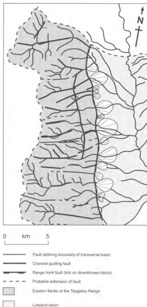
Fig. 6. The relationship between faulting and the location of transverse drainage systems and piedmont fan systems along the Taygetos range front.
