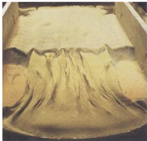
Fig. 11. Oblique view of the brittle-ductile interface (in foreground) of Experiment #27, after removal of upper granular layer (in background) with a vacuum hose. The width of the model between the vertical pistons is 9.6 cm. Strong vice ductile crust is pink, weak ductile crust is yellow.
