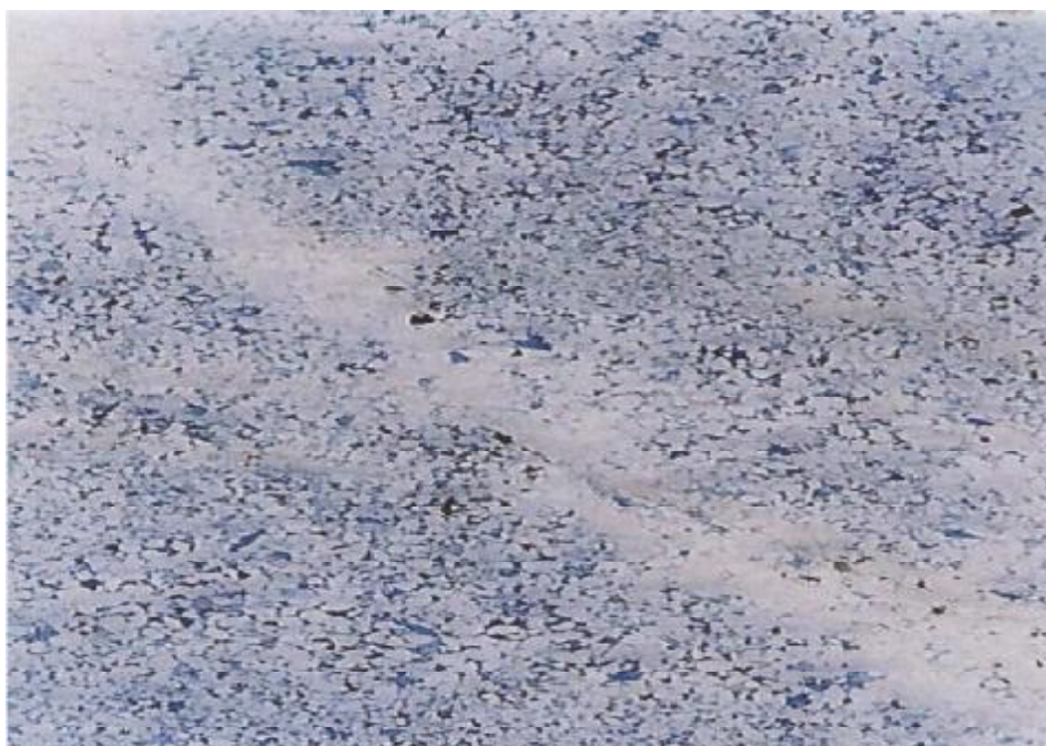
Scanned image of thin section of impregnated Sandstone (Garn Fm 4.8 km depth) from Haltenbanken. The shear bands are characterized by low porosity. (Cross section -3 cm)
