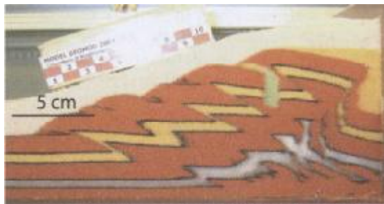
(f) Toronto – section close to sidewall (sidewall with foil)
