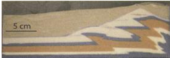
Fig. 6. Influence of lateral shear stresses illustrated in models of Parma (a–e) and Toronto (f and g). Structures are shown after 14 cm displacement. This model of Parma shown is with Alkor foil attached to the sidewalls (and is, therefore, different from the model in Fig. 2). The model of Toronto also has Alkor foil applied to the sidewalls (same model as in Fig. 2). (a) Cross section as observed through glass sidewalls. Note that Alkor foil partly obscures model visualization. (b) Cross section at 0.5 cm from sidewall. (c) Cross section through centre of model. (d) Contour map showing topography of deformed model, obtained by laser scanner; scale in cm above model base. (e) Topographic profiles 0.5 cm from sidewalls (right and left section) and through centre of model ('mid section'). (f) Cross section close to lateral sidewall. (g) Cross section through centre of model. Note that in (b), (c), (f) and (g) a sand layer was added on top of the model before cutting.
