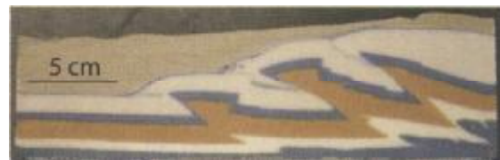
Fig. 6. Influence of lateral shear stresses illustrated in models of Parma (a–e) and Toronto (f and g). Structures are shown after 14 cm displacement. This model of Parma shown is with Alkor foil attached to the sidewalls (and is, therefore, different from the model in Fig. 2). The model of Toronto also has Alkor foil applied to the sidewalls (same model as in Fig. 2). (a) Cross section as observed through glass sidewalls. Note that Alkor foil partly obscures model visualization. (b) Cross section at 0.5 cm from sidewall. (c) Cross section through centre of model. (d) Contour map showing topography of deformed model, obtained by laser scanner; scale in cm above model base. (e) Topographic profiles 0.5 cm from sidewalls (right and left section) and through centre of model ('mid section'). (f) Cross section close to lateral sidewall. (g) Cross section through centre of model. Note that in (b), (c), (f) and (g) a sand layer was added on top of the model before cutting.
